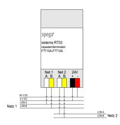
The LON repeater sistema RT-33 allows the increase of the number of participants or the communication range of the network. The required operating voltage is 24 V DC.
