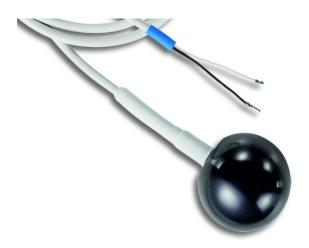
Sensor for detection of operative temperature (from mean Air and radiant temperature) in large rooms. Designed for direct connection to the multisensors lumina MS4 and lumina MS4-RC.
