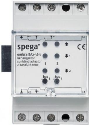
The ombra BA2-3E sunblind actuator can be used for sunblinds with 3 stop positions.
