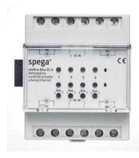
The ombra BA4-DC sunblind actuator is designed for connection to spega M/R series LON controller. The maximum switching capacity for each DC-motor is 1A.
